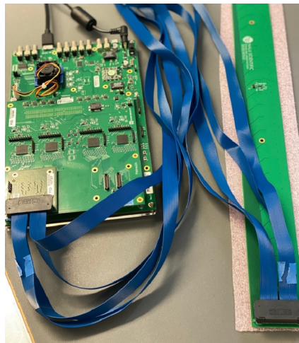
FIGURE 6: CAEN DT5550 readout connected to the muon board with SiPMs.
