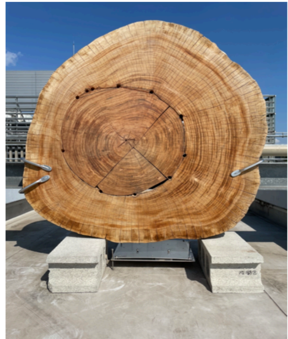
FIGURE 1: A cavity of approximately 50 cm was created in a 1.2-m-diameter wooden plate, and a nuclear emulsion detector was installed at the bottom of the wooden tree, to measure the difference in cosmic ray muon flux with and without the cavity.
