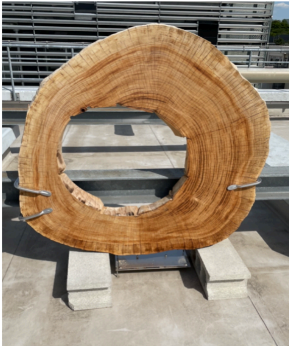
FIGURE 1: A cavity of approximately 50 cm was created in a 1.2-m-diameter wooden plate, and a nuclear emulsion detector was installed at the bottom of the wooden tree, to measure the difference in cosmic ray muon flux with and without the cavity.
