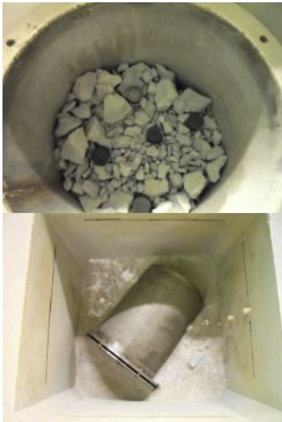
(a) The steel top hat with grout and uranium pennies inside
