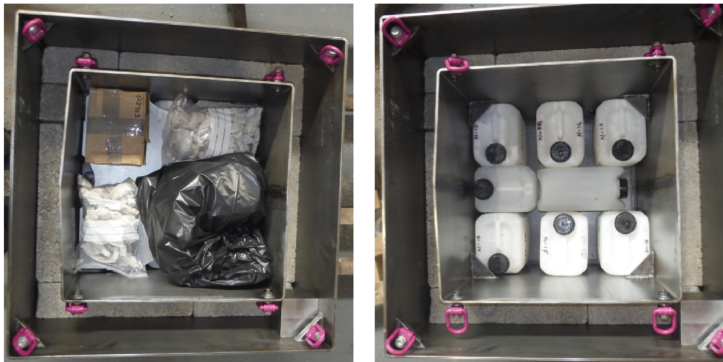
FIGURE 5: A small-scale version of a 3 m 3 box showing the top layer (left) of heterogeneous wastes and (right) the bottom layer with six jerry cans of simulant corroded sludge and the top layer. Also visible is the concrete liner and the 1 cm deformation of the left-hand wall of the inner skip.
