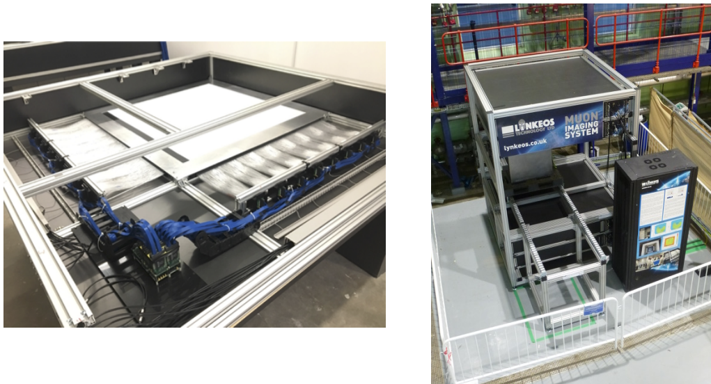
FIGURE 1: The interior of a tracking module showing the x - y grid of scintillating fibers (left) and the front-end readout, and the Lynkeos Muon Imaging System at NNL Central Laboratory (right).
