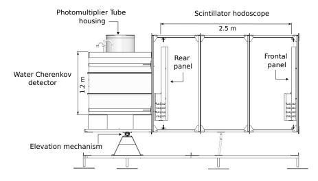
FIGURE 2: MuTe lateral view. The WCD, placed behind the scintillator hodoscope, measures the deposited energy of particles traversing the MuTe. The hodoscope measures the time of flight and reconstructs the trajectory of the impinging particles. The separation distance between the hodoscope panels varies from 40 cm up to 250 cm.
