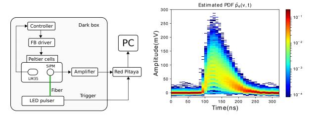
FIGURE 5: (Left) Experimental setup for measuring the gain and noise of the SiPM S13360-1350CS. A 480 nm pulsed light 10 ns width at 500 Hz stimulates the SiPM. The SiPM pulses are digitized at 14-bit/125 MHz. (Right) SiPM pulse waveform quantization.
