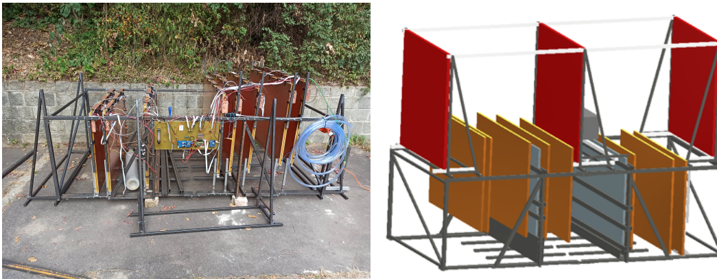
FIGURE 4: Detector system compatible with volcanology application, planned to be applied at Etna. The left panel shows the image of the MWPC tracking system, the right panel shows the full proposed setup with a scintillator telescope on top.
