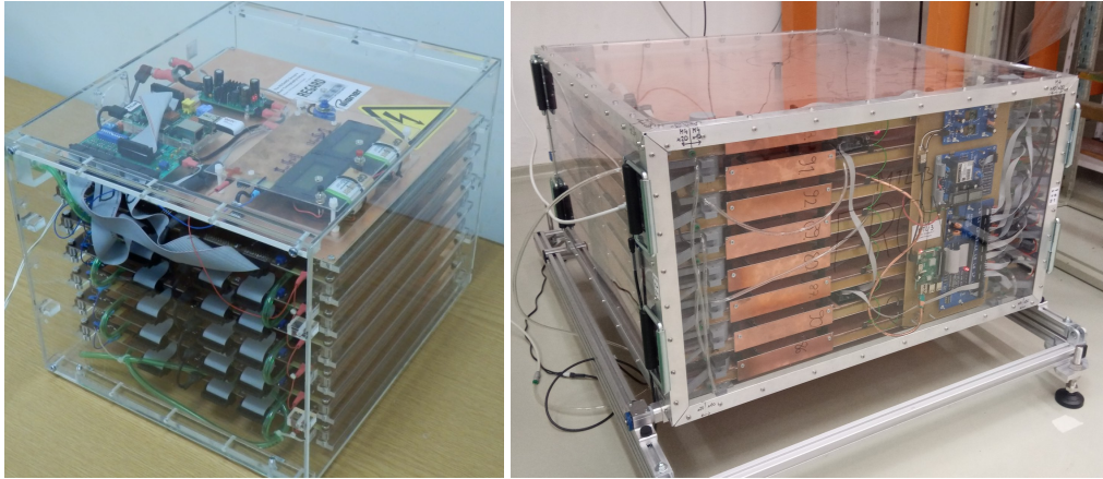
FIGURE 3: Left image: 25 cm size CCC-based compact tracking system. Right image: the “Muon Tomograph Large” version, with 76 cm by 76 cm sensitive area.
