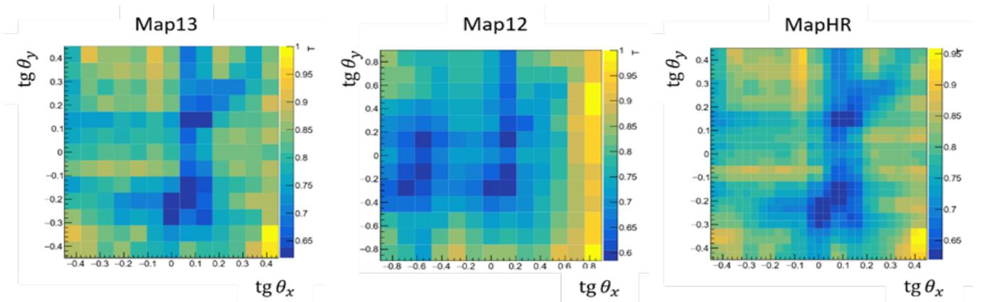
FIGURE 6: Example of the application of an iterative method to attain higher-resolution maps to a set of data acquired by the LouMu at the Physics Department of the University of Coimbra: (Left) Transmission Map13, (Center) Transmission Map12, and (Right) Transmission Map HR.
