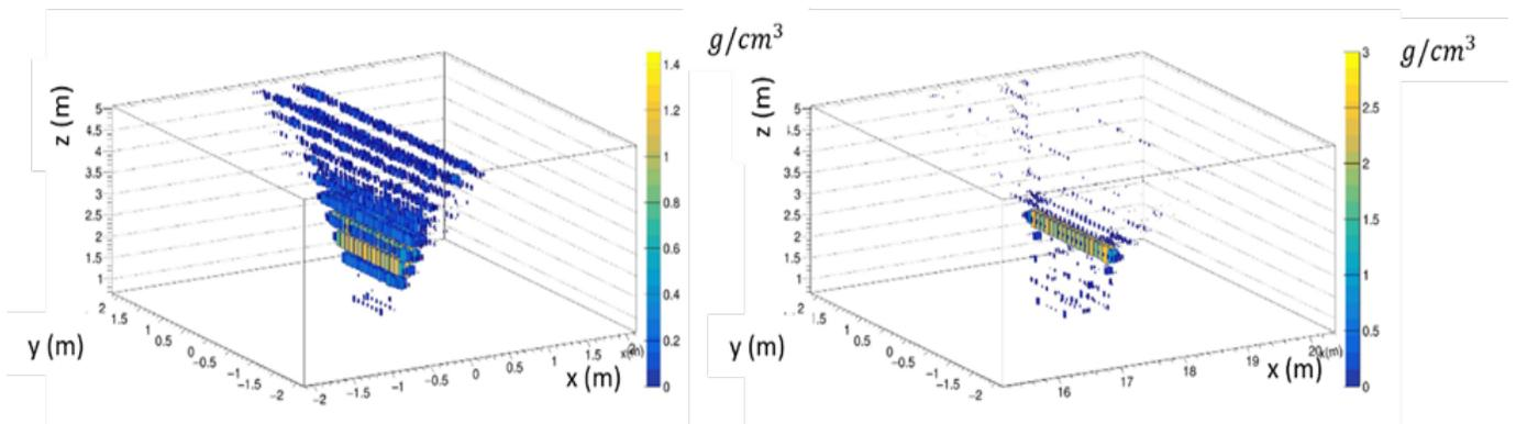
FIGURE 8: Results of the iterative reconstruction of a beam placed at 2.6 m height. (Left) Using one telescope position. (Right) Using three telescope positions.
