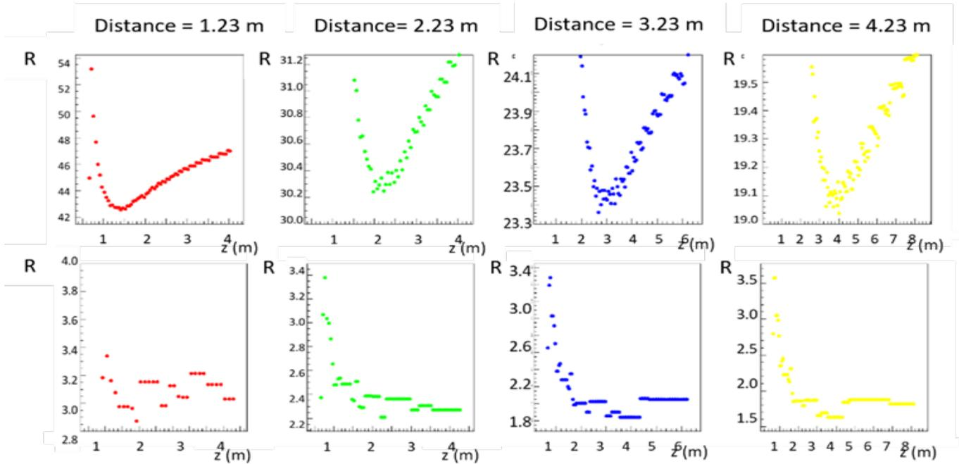
FIGURE 7: Plots of the angular width of the signal region ( $R$ ) versus the distance from the telescope ( $z$ ) for 4 different beam positionings relative to the telescope. (Top row) Using 10x LouMu's resolution. (Bottom row) Using LouMu's resolution.
