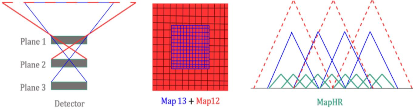
FIGURE 5: (Left and Center) Superposition of Map13 and Map12 fields of view. (Right) Schematics of the contribution of the values of Map13 and Map12 for MapHR.
