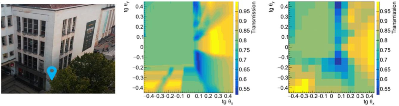
FIGURE 3: (Left) Location of the telescope used for the simulation results exemplified. (Center) 2D Transmission map simulated with 10x LouMu's resolution. (Right) 2D Transmission map simulated with LouMu's resolution.
