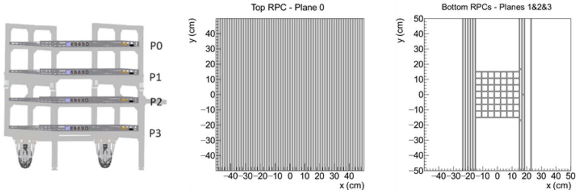
FIGURE 1: (Left) CAD of the LouMu telescope. (Center) Pad configuration of the top RPC. (Right) Pad configuration of the bottom RPCs.
