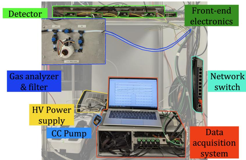
FIGURE 1: Image of the new version of the MUST<sup>2</sup> detector and peripherals.
