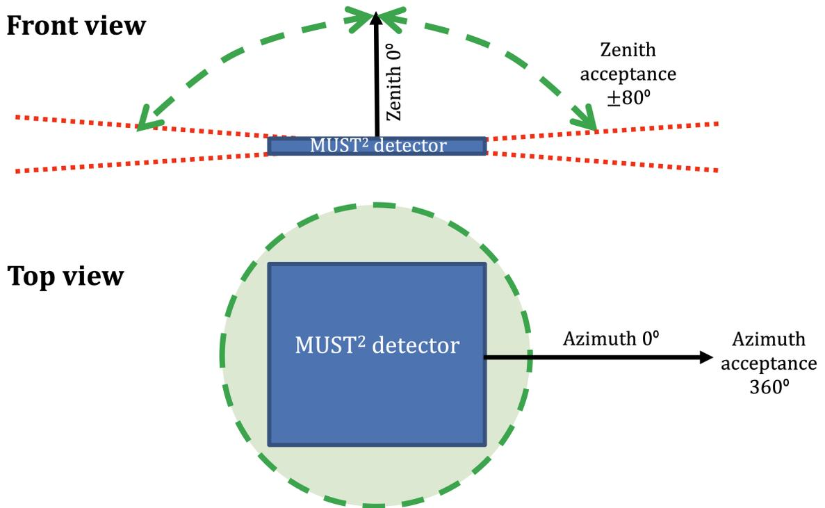
FIGURE 2: Diagram of the zenithal and azimuthal acceptance angles of MUST<sup>2</sup> detector.
