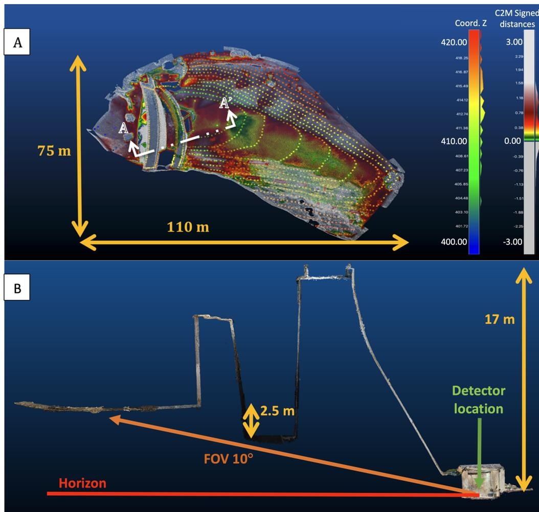
FIGURE 3: Model of the *Saint-Saturnin-lès-Apt* dam system, (A) top view and (B) detail of section A-A' with the location and field of view of the detector.
