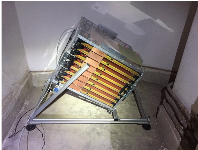
FIGURE 2: "Mts50" MWPC type detector with 50 \times 50 \text{ cm}^2 active area in tilted measurement position.
