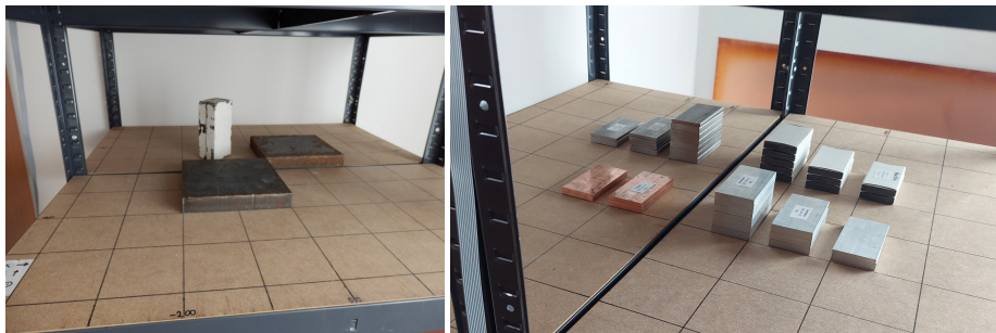
FIGURE 3: In the first measurement, 2 iron (25 mm each) and a lead (150 mm) brick were tested; in the second, iron (65, 30, 15 mm), lead (60, 30, 20 mm), aluminum (55, 30, 15 mm), and copper (15, 10 mm) were tested.
