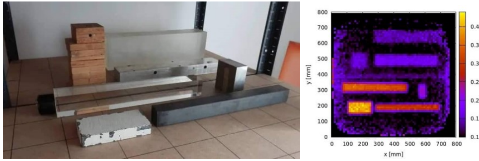
FIGURE 2: A picture and the 2D scattering strength map using various samples: lead brick, iron rod, lead glass scintillator, aluminum brick, aluminum rod, wood, and a plastic scintillator.
