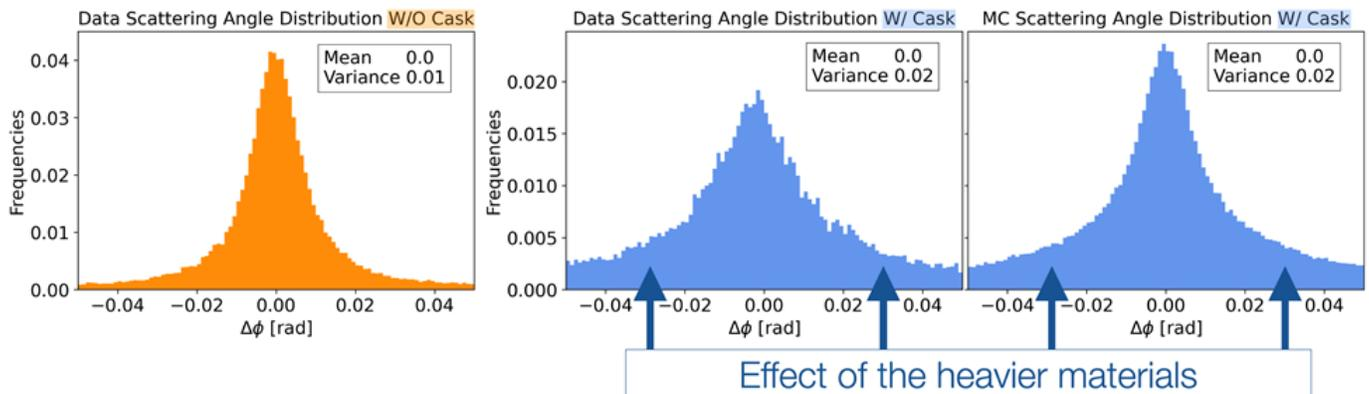
FIGURE 6: The reconstructed effective scattering angle distribution, measured without (left) and with (center) a fully loaded cask, and a comparison to the Monte Carlo simulation (right).
