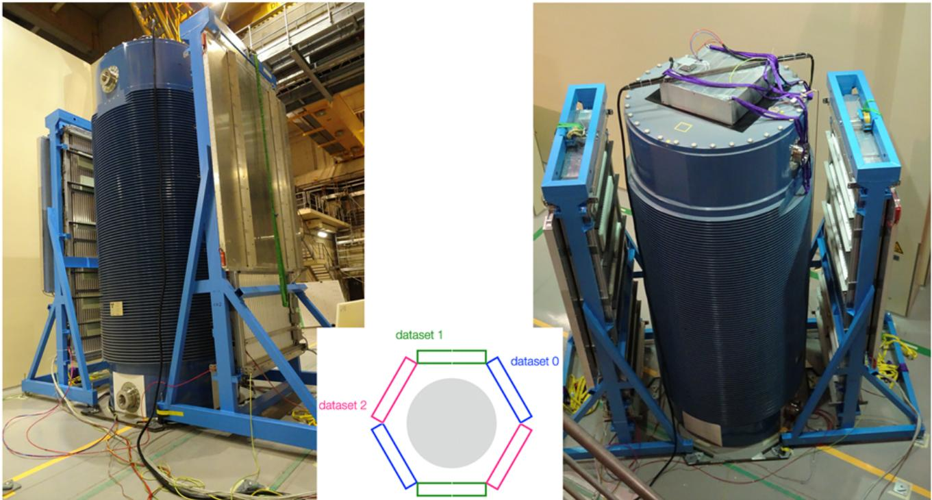
FIGURE 5: Photos of the Grafenrheinfeld field test installation. The detector, the support structure, and the CASTOR®V/19 cask are shown. The position of the detector modules during the data taking is summarized in the central graphic.
