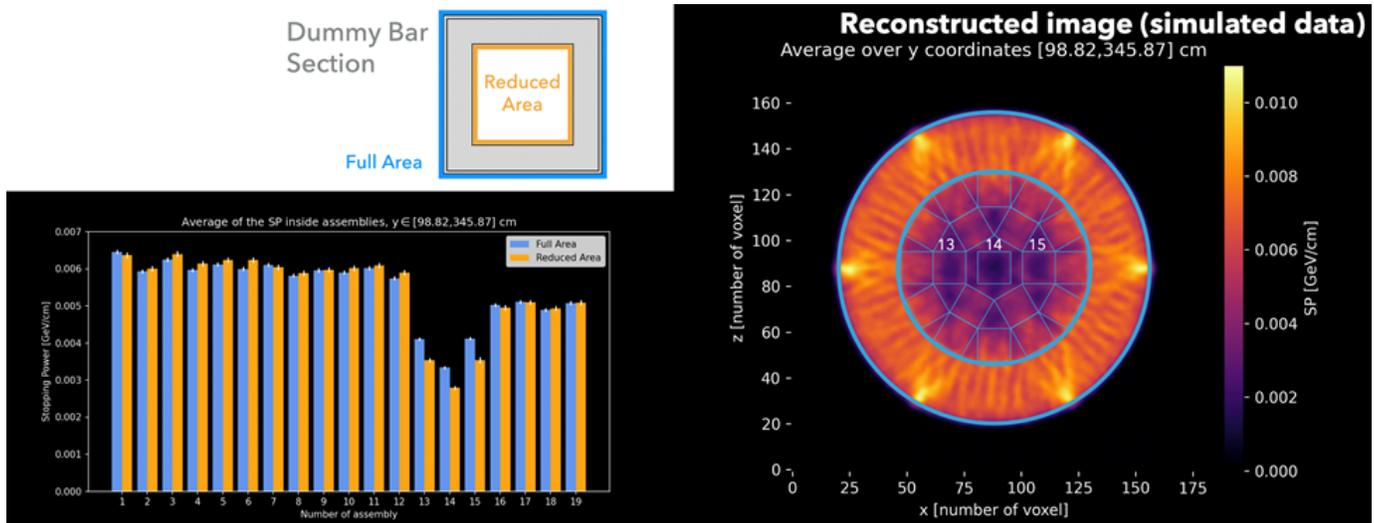
FIGURE 4: Left: a diagram showing the average of the SP inside assemblies can be seen. Right: example of a reconstructed image of a simulation of a CASTOR<sup>®</sup>V/19 cask with three dummy elements corresponding to position numbers 13, 14, and 15. The image has been obtained using the absorption algorithm.
