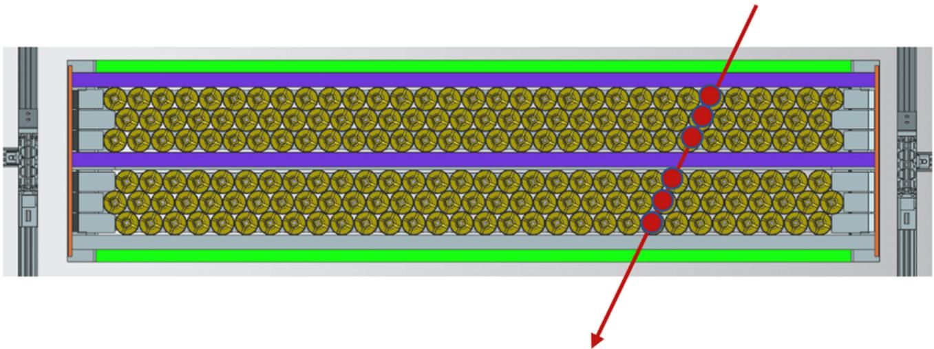
FIGURE 1: Top view of a drift tube muon detector module. The circles represent the Drift Tubes. The red arrow shows an example of a possible muon track crossing the tubes.
