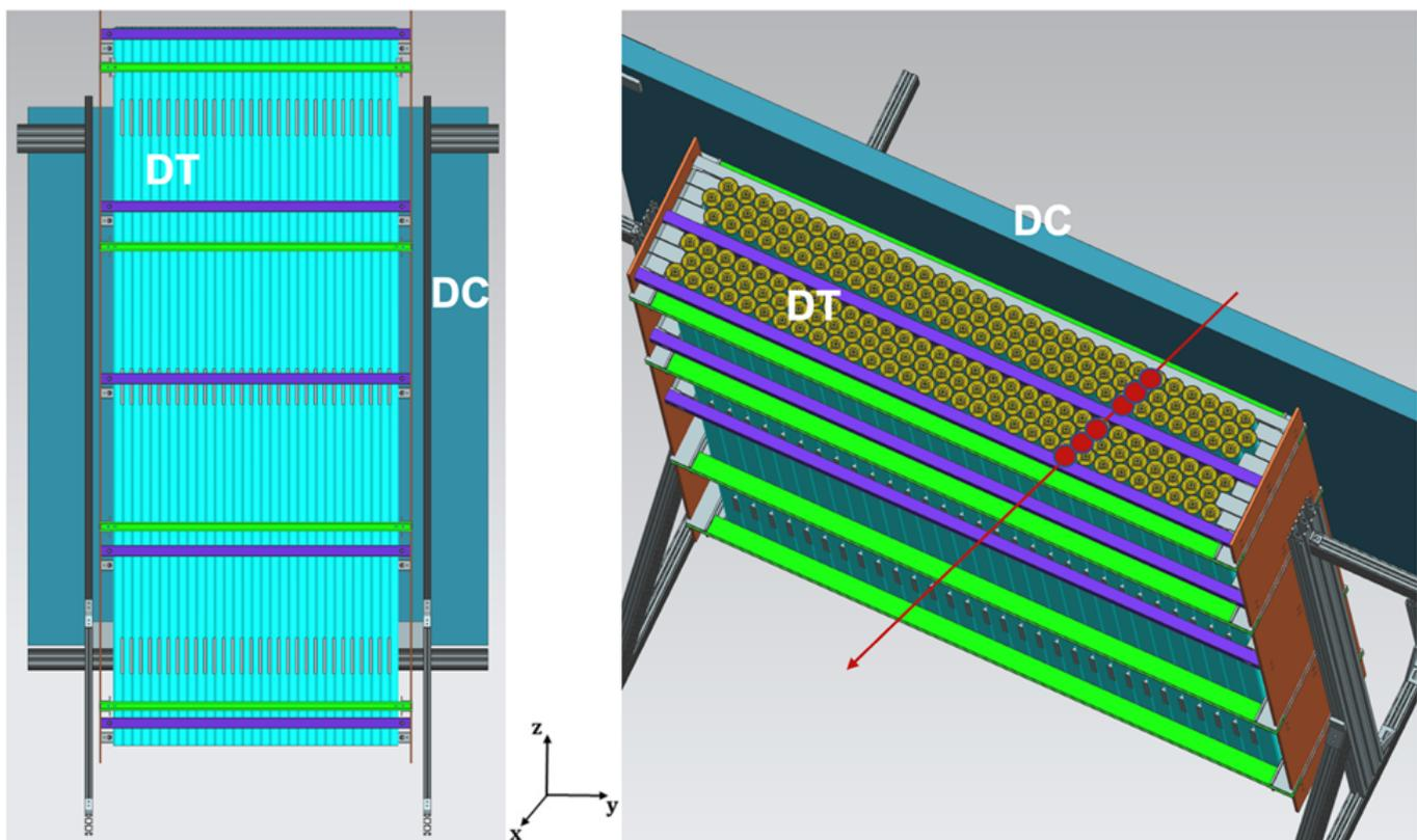
FIGURE 2: Scheme of the overall experimental detector apparatus including the INFN Drift Cells (DCs) and rectangular blue object attached on the back of the Drift Tubes (DT) modules. Left: one detector module in the  $z$ - $y$  plane. Right: top view with an exemplary muon track hitting the tubes (red).
