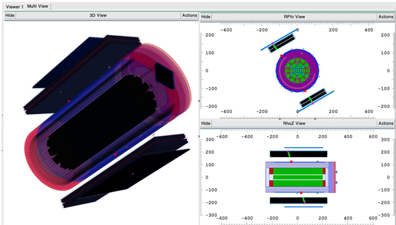
FIGURE 3: The figure shows a screenshot of the program used for visualizing the MUTOMCA Monte Carlo simulation including the CASTOR<sup>®</sup>V/19 and the detector modules. Additionally, one generated cosmic-ray muon track is shown (red, pink, and green dots).
