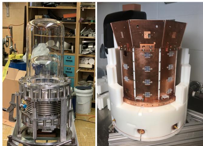
FIGURE 4: Left: view of the active area of SBC with the fused silica vessels connected by a bellows. Right: mounts for the SiPMs which surround the active area of SBC. Taken from [19].
