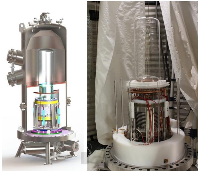
FIGURE 3: Left: a schematic view of the PICO-40L detector. Of particular note are the nested jars containing the target material and connected by a bellows. Right: a picture of the PICO-40L detector during construction. Taken from [18].
