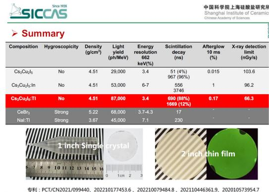
**FIGURE 11:** The R&D works on new Cs-Cu-I based crystals by SIC group [43].
