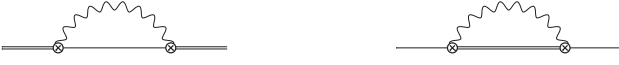
FIGURE 1: (Left) One-loop self-energy diagram of a scattering state (double solid line) in pNRQED DM ; the imaginary part is related to the bound-state formation process (X\bar{X})_p \rightarrow \gamma + (X\bar{X})_n . (Right) One-loop self-energy diagram of a bound state (solid line); the imaginary part is responsible for the bound-state dissociation process \gamma + (X\bar{X})_n \rightarrow (X\bar{X})_p . The cross circled vertex denotes the electric dipole interaction in equation (5).
